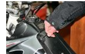
REMOVE THE UPPER MOUNTING BOLTS OF THE FRONT FAIRINGS.
