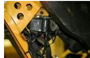
REMOVE THE ORIGINAL HV COIL DISCONNECTING CORRESPONDANT WIRES.
