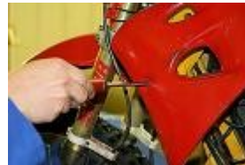
REMOVE THE ORIGINAL HV COIL DISCONNECTING CORRESPONDANT WIRES.
