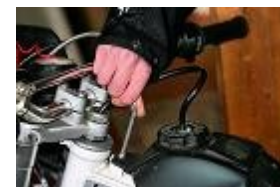
ONCE BOTH FRONT FAIRINGS REMOVED, UNSCREW THE GASOLINE TANK TIGHTENING BOLT.
