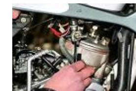
TURN THE GASOLINE TAP TO OFF POSITION AND REMOVE THE CONNEXION HOSE.
