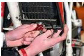
REMOVE THE LOWER MOUNTING BOLTS OF THE FRONT FAIRINGS.
