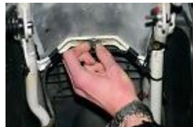
UNSCREW THE WING NUT UNDER THE SEAT.
