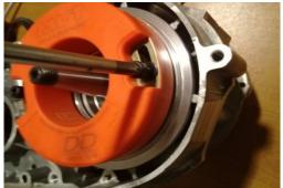
5- TIGHT MVT STATOR ON HIS BASE PLATE SETTING BOTH 5x30mm SCREWS AT THE MIDDLE OF THE ADJUSTMENTS RANGE.
