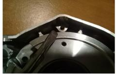
3-THIGHT MVT BASE PLATE ON THE ENGINE WITH CORRESPONDANT DELIVERED BOLTS.
